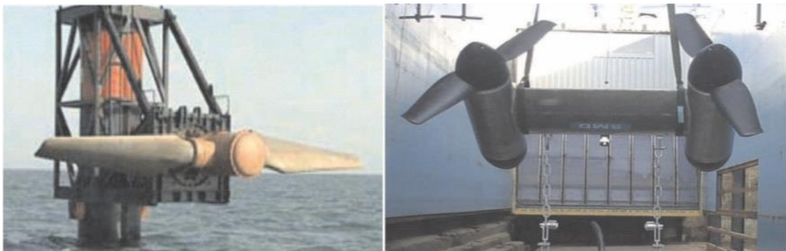
(a) Turbina de 300 kW, Marine Current Turbine (b) Turbinas de 500 kW, SMD Hydrovision
